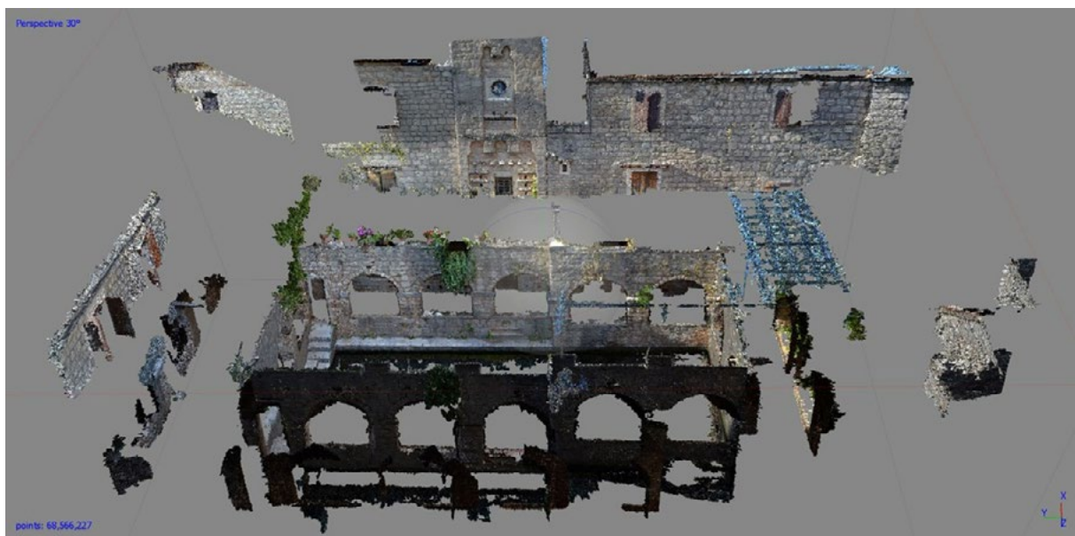
Fig. 1. Point of cloud made with photogrammetric representation software. Hvar Tvrdalj Fortress.
