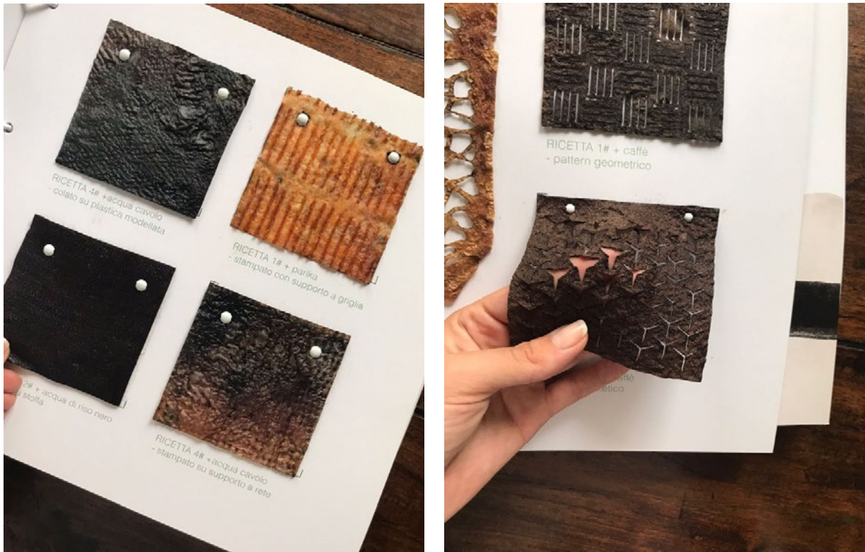
Fig 2. Alginate Materials Samples Collection: textures & patterns Collection (Credits: Giulia Colarieti, Supervisor: Sabrina Lucibello, Co-supervisor: Lorena Trebbi)
